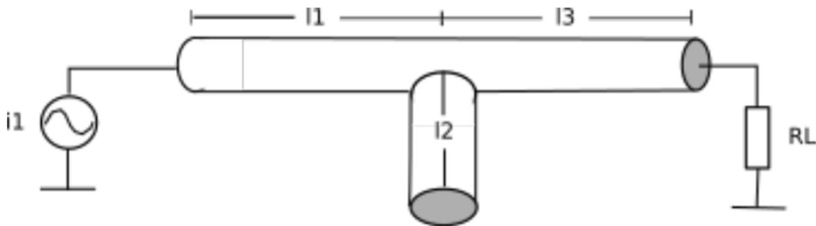
At the wavelength  $\lambda = 4l_2$ , there is a destructive interference leading to zero impedance in parallel with  $R_L$  and the segment of length  $l_3$ .
