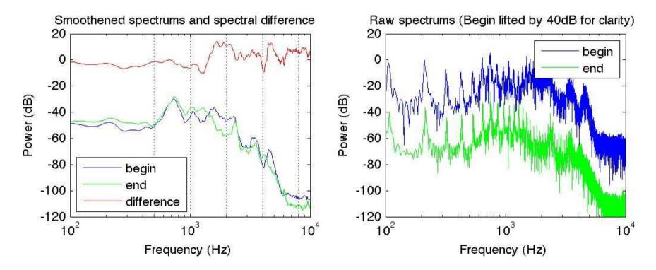
Spectra of vowel [ae] at 110 Hz, 8 s scan.
