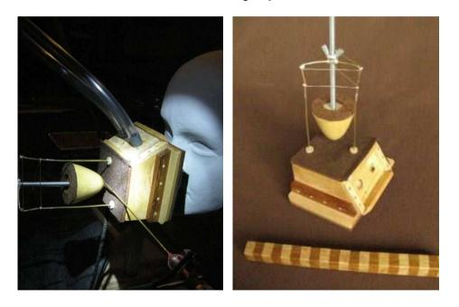
As shown on the right, the noise collector beam is widened by shadowing it with a paraboloid in front.
