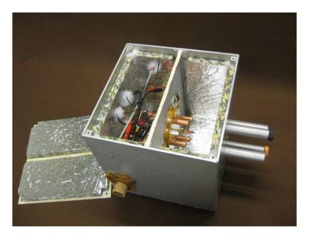
The speech and noise signals are then taken to an adjustable differential amplifier using RF-shielded cables.
