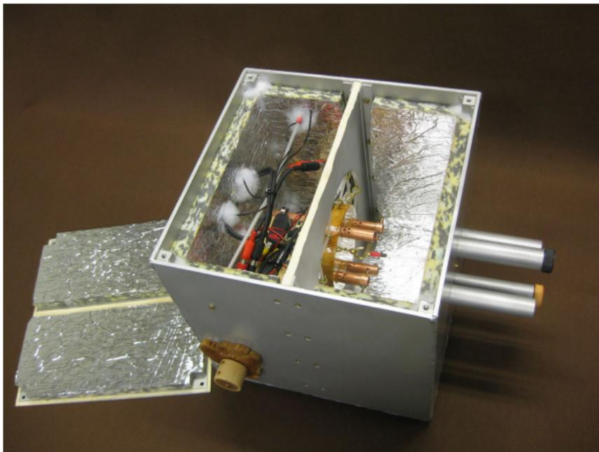
The waveguides lead to a microphone assembly inside a sound-proof Faraday cage, beside the MRI scanner.
