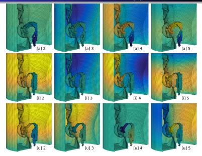
Resonant sound pressure fields of [a], [i], [u] in a constrained environment.
