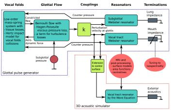
DICO is an interconnected network of mechanical, flow-mechanical and acoustic partial models.
