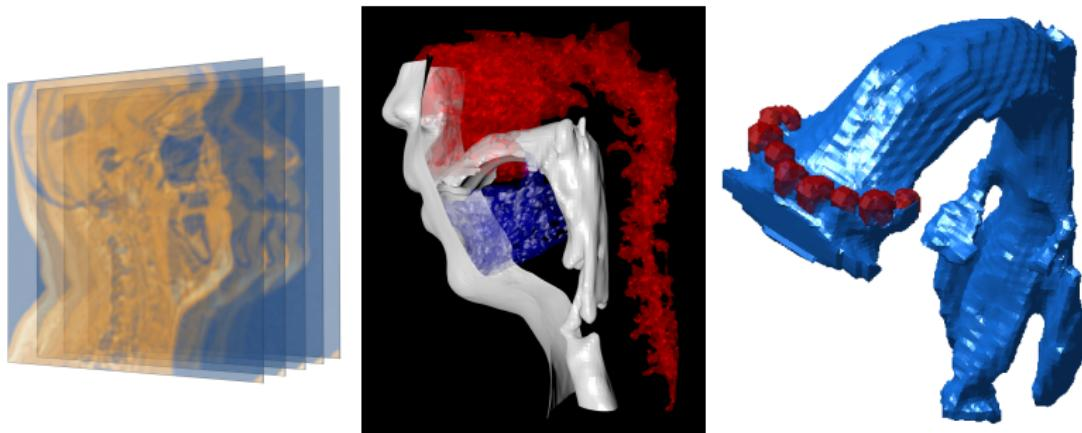
To solve acoustic equations, the surface models need be further processed to Finite Element Meshes.
