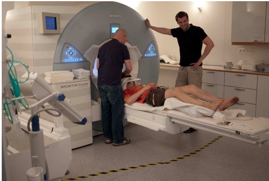
Figure 4.1: Test subject and equipment under preparation for the first recordings. Dr. Tech. Jarmo Malinen (left) is placing the sound collector on the MR registering coil over the face of the test subject (middle) while Dr. Jani Saunavaara (right) is observing.
