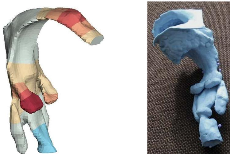
**Figure 1.3:** A surface mode of a pressure distribution for the 5th resonance of vowel [e] and a 3D print of the geometry for vowel [a].
